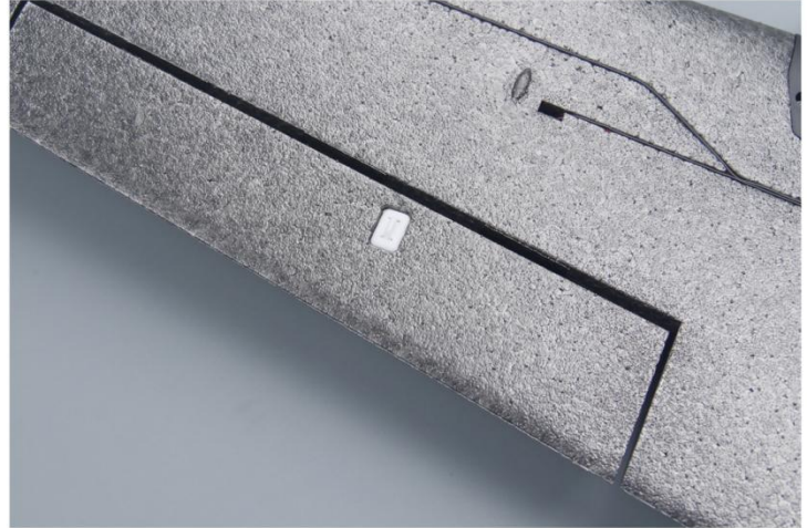
On the reverse side, install the horn buckle and recommend to apply some glue to secure.
