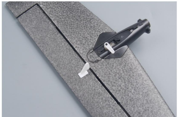
Install the horn chuck onto Horizontal tail as same way as aileron.
