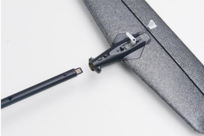
Install the horizontal tail.
