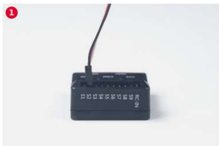
① connection to output S2 · ② ESC connection
