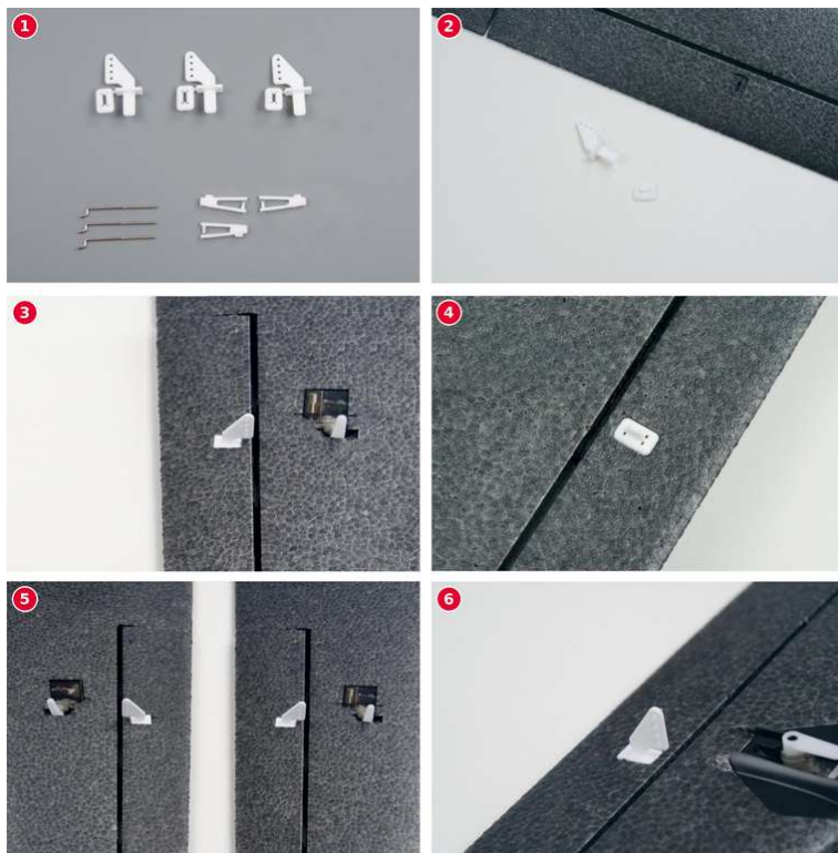
Installing the control horns ① to ⑥
