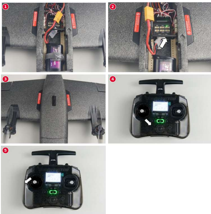
Power-on ① to ③, Arm ④ and Disarm ⑤
