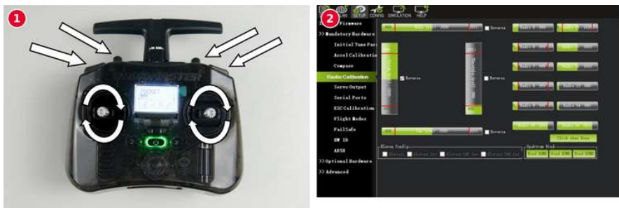
① moving the sticks and switches · ② response in Mission Planner
