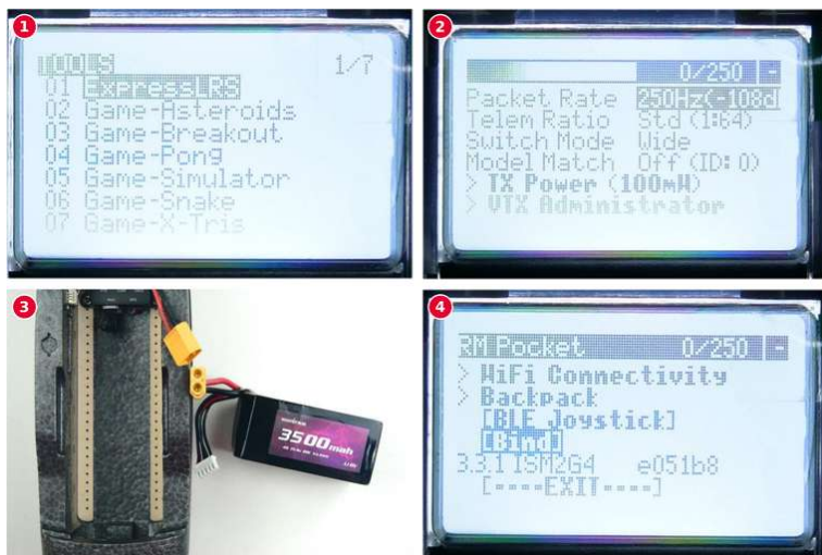
Steps ① to ④ of ExpressLRS receiver binding
