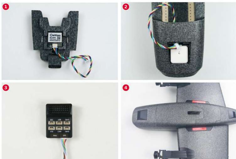
Installing the GPS module ① to ④
