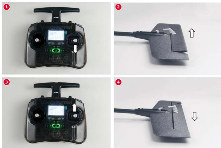
Elevator check ① to ④
