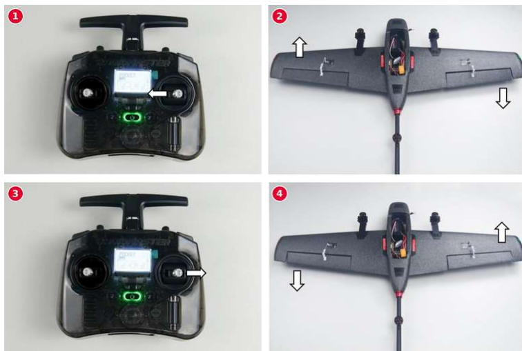
Aileron check ① to ④
