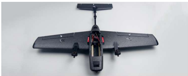
Servo horn and linkage installation completed
