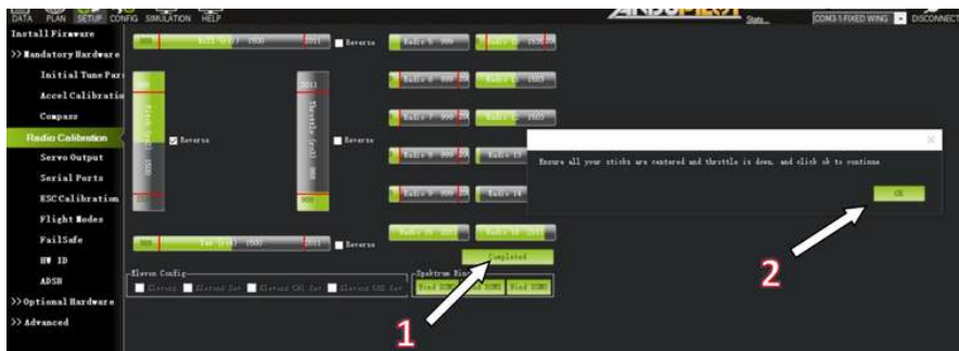
Completing the calibration, steps 1 and 2
