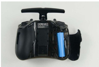
Position of the 18650 batteries in the Pocket radio
