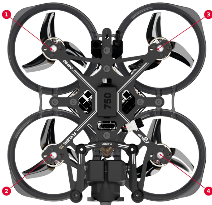
Motor numbering seen from above. The camera points towards the bottom of the picture.
