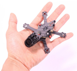
Example of a quadcopter built on the Cub-AIO frame. Electronics, motors and camera are not included.
