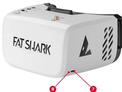
Side view – charging port
