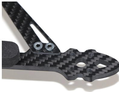
Brace-to-arm joint – two screws with lock nuts
