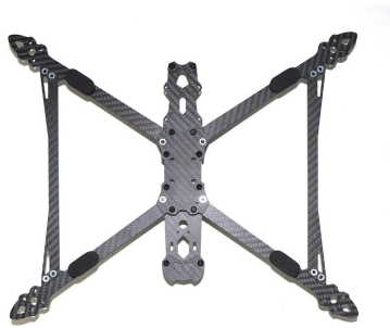
Bottom view of the assembled arms with braces and foam pads
