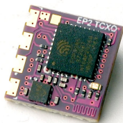
Side with the ESP8285 processor and the EP2 TCXO marking
