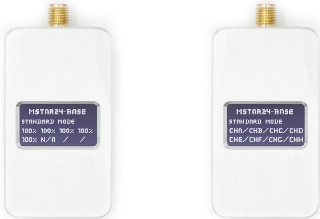
The ground module display: channel signal strength and the ChA-ChH channel assignment
