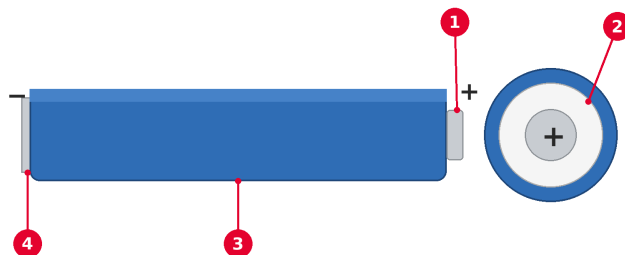
Fig. 1 – Cylindrical cell: ① positive terminal (+), ② insulating ring, ③ shrink wrap (sleeve), ④ negative terminal (–)
