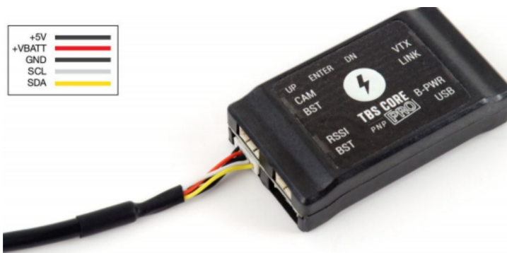
BST cable pinout: +5V, +VBATT, GND, SCL, SDA (Nano RX uses only GND, SCL and SDA)
