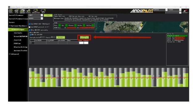
In the RTCM box it shows that the base status indicator is green and both the GPS and Glonass satellite systems are green (if you want to change the satellite system, refer to the following section). The box on the right says "Position is valid".
