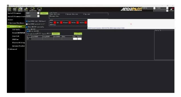
Select the correct base module com port in the top left corner and click connect. In the SurveyIn Acc section, enter the absolute geographic accuracy that you expect your Here 4 Base station to achieve. In the Time column, enter the minimum survey time you expect. Click on Restart, the ground station will transfer the data you have entered to the Here 4 base module, the base module will start a new round of surveying. You will see the following page:
