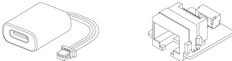
Left: J1.0 Config Module. Right: Network Conversion Module.
